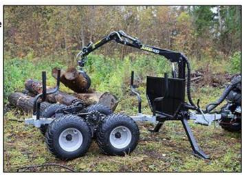
better-protected 4WD system, which is available now in two versions (200cc and 400cc). Off course there are swinging tandem axles, heavy duty 8 ply tires and swivel towing hitch. For the crane and timber trailer can be added a variety of accessories for expanding the use of it. Hydraulic tipping box, remotely operated hydraulic winch, telescopic extension for the crane, earth bucket, earth drills, energy wood head, etc ...
